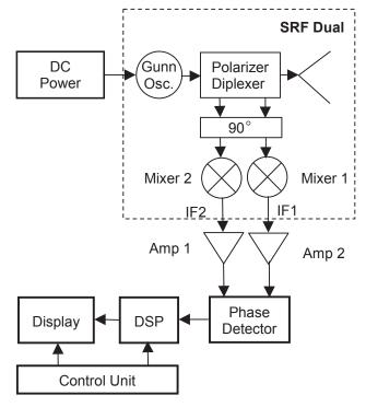
Figure 3. Simplied Directional Doppler Radar
