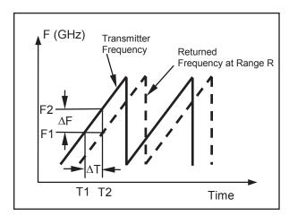
Figure 5. FMCW Radar Frequency vs. Time
