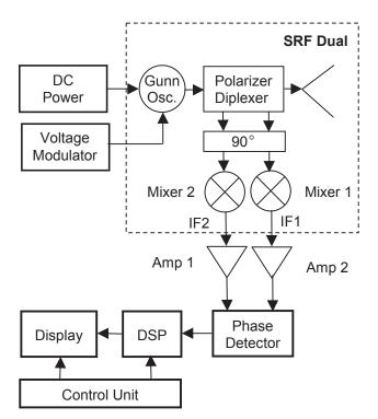
Figure 6. Simplied FMCW Ranging Radar with Directional Doppler Feature
