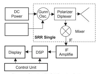
Figure 4. Simplied FMCW Ranging Radar
