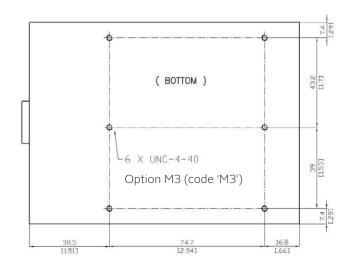
Maximum lenght of the fastening screws : For UNC-4-40 : 0.1968'' For M3 : 5 mm
