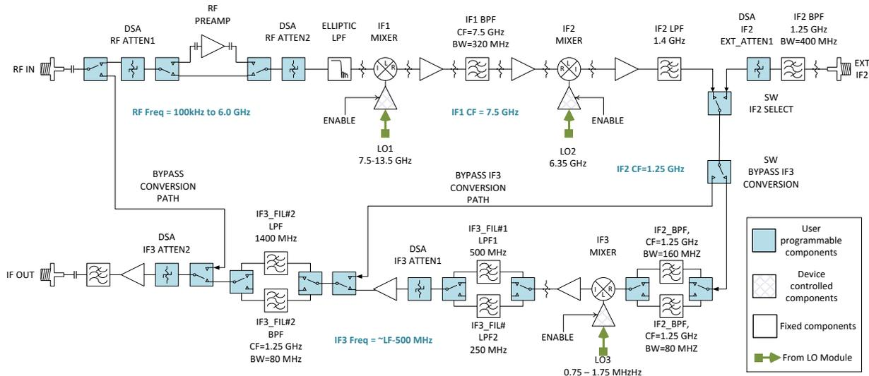
Figure 4. Block diagram of the signal conversion module of the downconverter assembly
