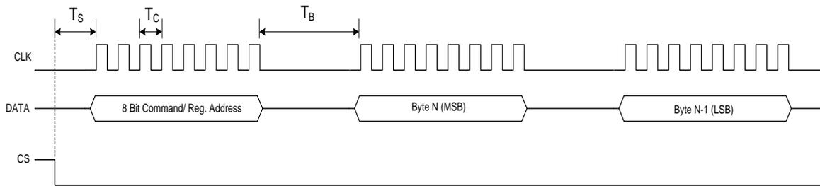
Figure 9. SPI timing.
