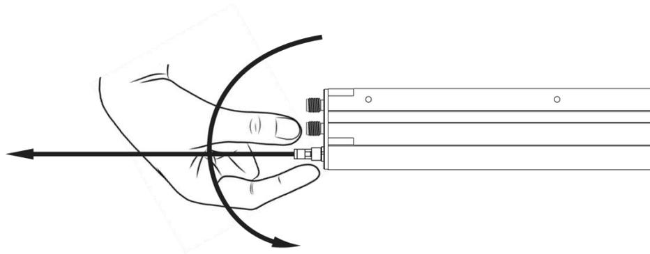
Figure 2. Proper Removal of Latching-Style Ribbon Cable Connectors
