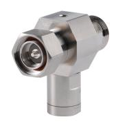
Arrestor Plus® Dual Band Quarterwave Surge Arrestor (T-shaped), 806–960 MHz and 1700–2170 MHz, with interface types DIN Female Bulkhead and DIN Male
