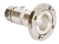
1-5/8 in EIA Female Flange for 7/8 in HJ5-50 air dielectric cables. Includes gas barrier that can be drilled in predetermined location for gaspass.
