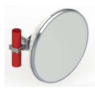
0.9m | 3 ft ValuLine® High Performance Low Profile Antenna, single-polarized, 5.925–7.125 GHz, PDR70 flange, white antenna, composite broadband grey radome without flash, standard pack—one-piece reflector
