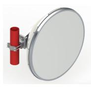
0.9m | 3 ft ValuLine® High Performance Low Profile Antenna, dualpolarized, 5.925–7.125 GHz, PDR70 flange, white antenna, composite broadband grey radome without flash, standard pack—one-piece reflector
